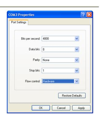
Once the HyperTerminal settings have been entered you should try pressing print on the scale/balance/indicator etc and hopefully you will see a reading appear in HyperTerminal like below (Note: the scale output varies considerably per model but as long as you can see something that resembles the reading from the scale it should be working, you may also see lots of extra information depending upon the model, that is not displayed on the scale's screen – that is ok).
