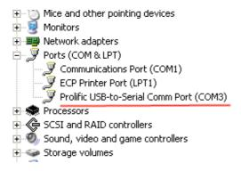
Note: the name of connection "Prolific USB-to-serial" in the above example varies per scale.
