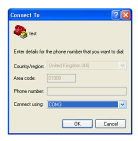
Set the com port to the virtual com port of your USB/virtual com port – COM3 in this example. Next set the Baud settings, typically 4800 Bps, 8 data bits, no parity and 1 stop bit for most ADAM scales (though not all, so you need to check the user manual's RS232 Section to find out how to check the settings inside your scale/balance.
