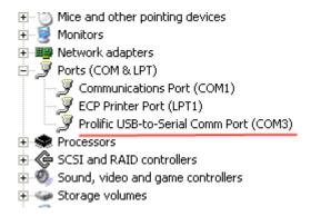
This should also list the virtual comport number it is using. If it does not show up under ports or there is a yellow exclamation symbol next to it then there is a problem with the driver or the physical device. Read the convertor's installation manual for help.
