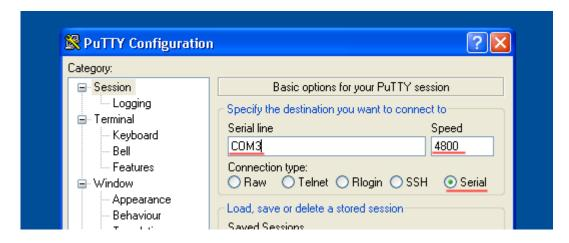
Next set the Baud/speed setting, typically 4800, 8 data bits, no parity and 1 stop bit for most ADAM scales (though not all, so you need to check the user manual's RS232 Section to find out how to check the settings inside your scale/balance. The flow control can be left at its default.
