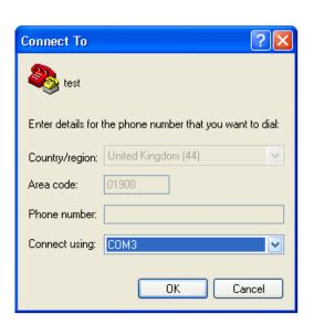
Set the com port to the virtual com port of your USB to RS232 convertor – COM3 in this example. Next set the Baud settings, typically 4800 Bps, 8 data bits, no parity and 1 stop bit for most ADAM scales (though not all, so you need to check the user manual's RS232 Section to find out how to check the settings inside your scale/balance.
